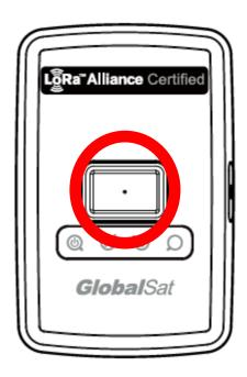
When help button is long pressed, LT-100 will send the first help report immediately. Then LT-100 would send help reports every 30 seconds (default value) continuously to LoRaWAN<sup>™</sup> gateway till it gets server acknowledgement and GPS fix.
