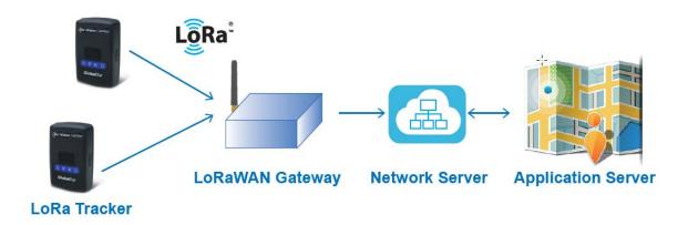
Before starting communication LoRaWAN<sup>TM</sup> gateway and LT-100 LoRa<sup>®</sup> trackers, please refer to the LoRaWAN<sup>TM</sup> gateway's user manual to set the LoRa<sup>®</sup> settings described on "4. LoRa<sup>®</sup> settings" by GlobalSat-LT-100 Config Tool.
