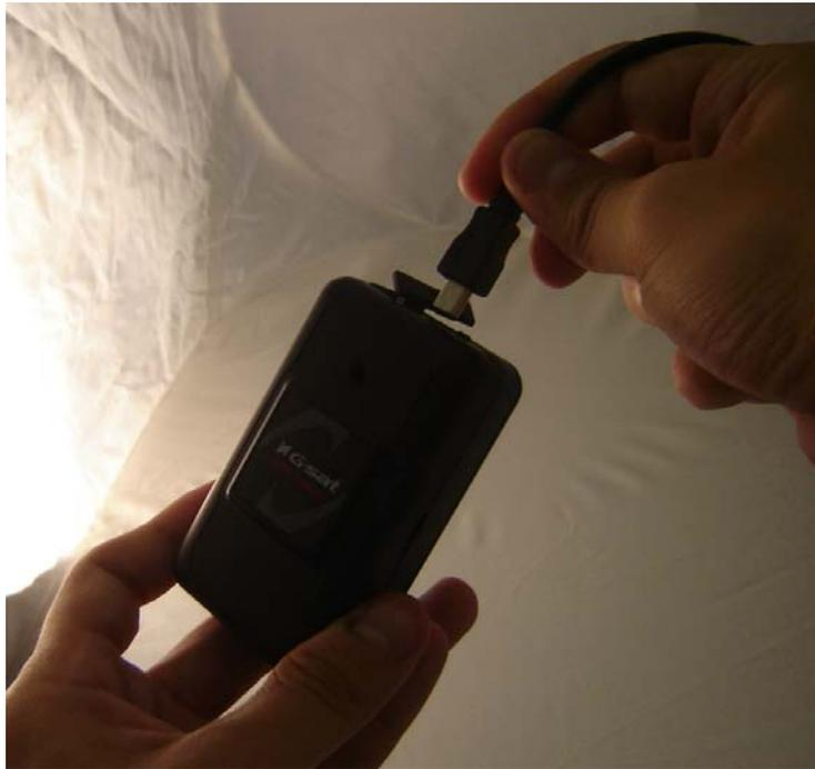
Before using TR-151 for the first time, please fully charge it by connecting to AC power adapter under the power-off condition. (The attached battery is specially designed for TR-151. Please do not use other type of battery; otherwise it will damage the device. If you need to change the battery of TR-151, please contact your local dealer.) You can also charge the TR-151 by connect it to PC or Notebook via USB cable. (The power of PC or of notebook should be turned on.)
